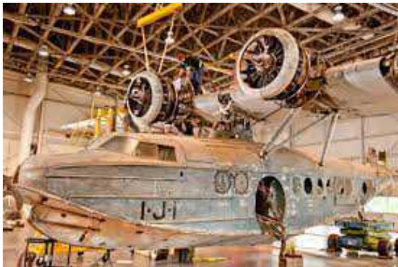
Mounting an engine in the Ruth Baker Engen Restoration Hangar at the Udvar-Hazy Annex.
