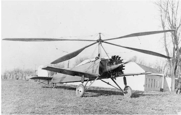
C.8W [powered by a 225 hp Wright Whirlwind]. (Credit: National Air and Space Museum)
