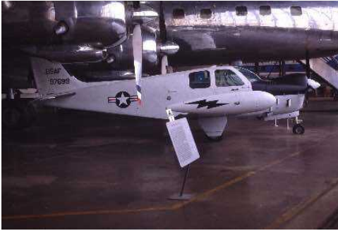
Note the bulged nose fairing needed to allow for installation of the heavy duty alternator required to run the electronics.
