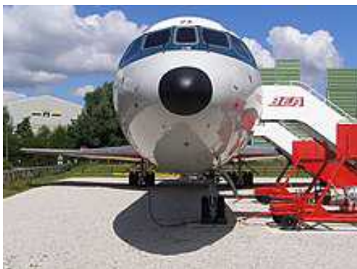
The Trident Off-Set Nose Gear (Credit: MilborneOne)
