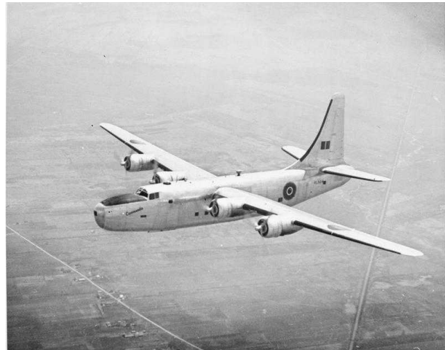
Commando. Note the single vertical tail which will be adopted by the PB4Y-2 Privateer. Credit: Brock F J (Fg Off), Royal Air Force Imperial War Museum
