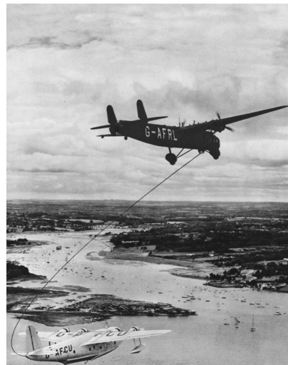
A Handley Page HP.54 Harrow refuels the Short Empire Flying Boat Cabot using a looped hose and grapple.
