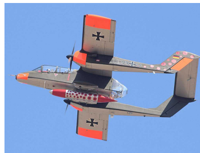
A Luftwaffe OV-10B target tow aircraft with the target operator in a greenhouse pod mounted in the aft portion of the nacelle. (Credit: Adrian Pingstone)
