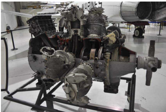
A cross-section RS-3350 indicating the complexity of the engine. Note the staggered arrangement of the two cylinder banks to improve cooling of the rear bank. Now imagine the tight cowling and its effect on air flow.
