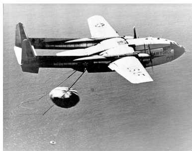
A trapeze equipped Flying Boxcar retrieving a capsule. (Credit: USAF)
