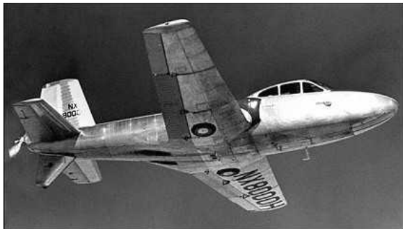
Note the tail skid to prevent prop strikes.
