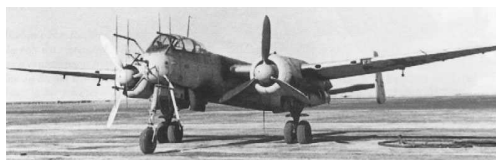
The Luftwaffe's other Uhu, a night interceptor sporting Hirschgeweih (Deer Antlers) VHF radar antennas.
