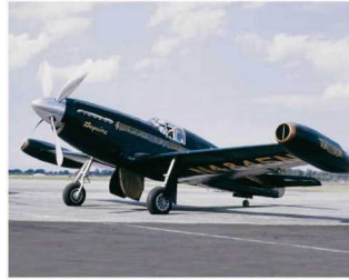
The jet-like pods on the wing are radiator and engine air coolers.
