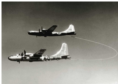
Lucky Lady II refueling from a looped hose on its circumnavigation of the globe. (Credit: USAF)
