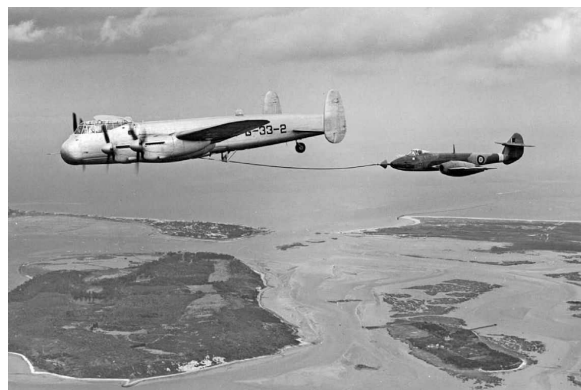
Modified Lancaster refueling Meteor with the probe and drogue. (Credit: Flight Refueling Ltd.)
