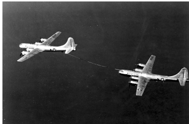
KB-29M in an early test refueling a B-29. (Credit: USAF)
