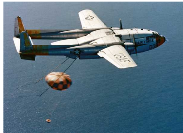
A successful retrieval of a re-entered camera and film pod. (Credit: National Reconnaissance Office)
