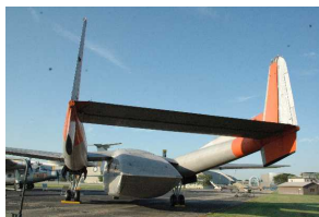
The "beaver-tail" hatch in both closed and open position.
