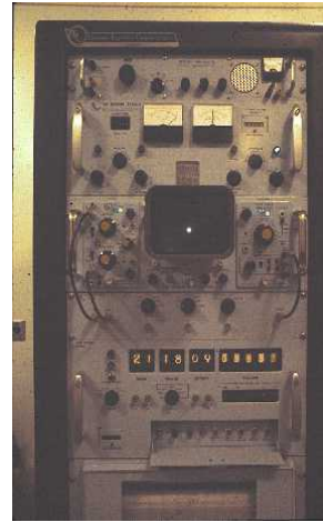
Clock and Laser Control Station. Note the five decimal point readout. The millionth second is read from the oscilloscope.
