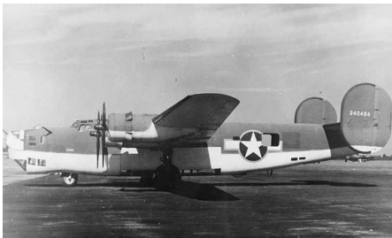
A modified B-24D The retracted antenna for the radar is visible aft of the open bomb bay doors in place of the ventral gun turret.
