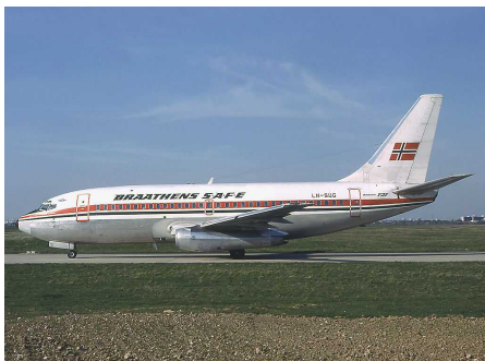
The early 737s with wingspans about equal to length were known as “Fat Alberts.” (Credit: Michael Gillian)
