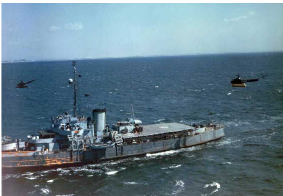
A U.S. Coast Guard Sikorsky HNS-1 helicopter (right) and a Sikorsky HOS-1 (left) conducting experimental flight operations on USCGC Cobb, 15 June 1944. (Credits: USCG)
