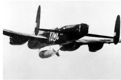
Lancaster releasing a Tallboy from its modified bomb bay. (Credit: Imperial War Museum.)
