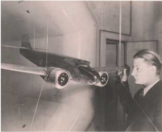
Johnson, testing the original single tail Electra in the University of Michigan wind tunnel.
