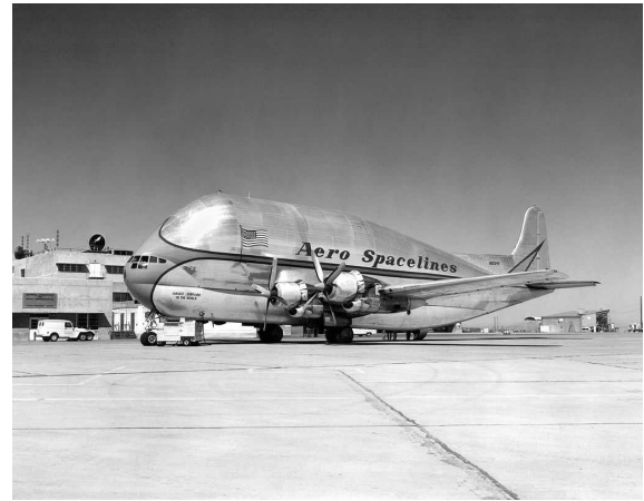
The Pregnant Guppy, an ex PanAm airframe with a five meter section from an ex-BOAC 377 inserted behind the wing.
