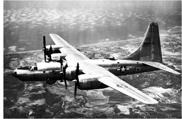
The production Dominators were built with the single high tail similar to those used on the Navy's Privateers.
