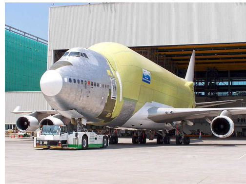
The first Dreamlifter with an initial green zinc chromate anti-corrosion coating is rolled out from the Evergreen hangar, Taoyuan International Airport, Taiwan.
