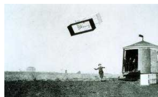
Kite reel house and kite with met instruments mounted.
