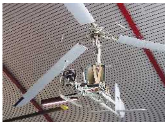
A Focke-Achgelis Fa 330 Bachstelze (Wagtail) towed by a U-Boat.
