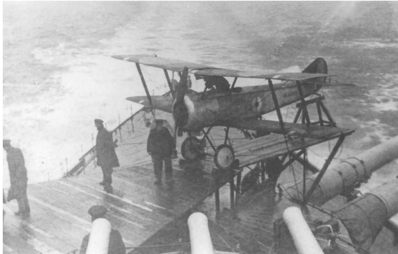
Sopwith Pup on platform. Note how a turret mounted landing platform will restrict the training and use of the naval rifles.
