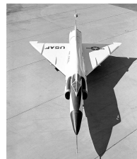
The “Coke Bottle fuselage indicating the application of the Area Rule is evident on this NACA Convair F-102A Delta Dagger.
