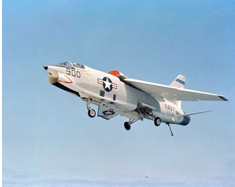
The windows for the four camera bays are visible just below the national insignia and on the belly. A forward looking camera looks through the protrusion just forward of the nose wheel.
