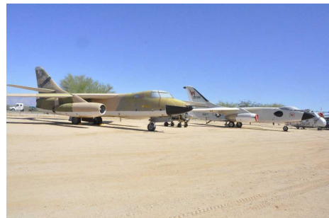
The B-66 Destroyer in the foreground is the USAF light bomber version of the Skywarrior in the background.
