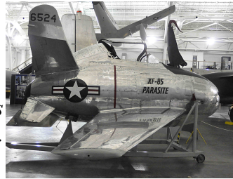
XF-85 Goblin, an attempt to develop a parasite fighter to be carried by a bomber as an escort when needed.
