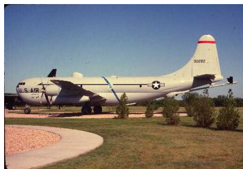
KC-97L at Dyess AFB sporting two J-47 auxiliary turbojets. 81 were built.
