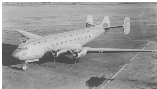
The triple tail allowed it to fit inside hangars then in use and provided more yaw control in an engine-out situation.
