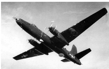
The Mercator has four engines. Two turbojets are mounted within the bottom of the engine nacelles.
