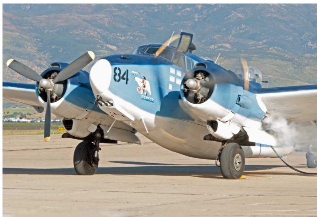
Attu Warrior, the only airworthy Harpoon. Note he heavy nose armament on the Harpoons.
