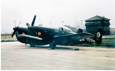
F-82G night fighter of the 68th F(AW)S as flown by Lt Hudson and Fraser. The protuberance between the twin fuselages housed the radar and associated electronics
